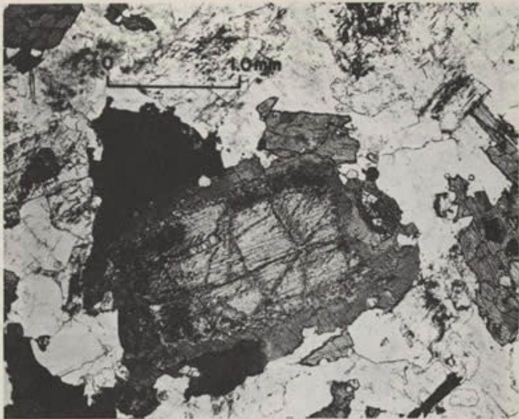
FIGURE 8. Large core of clinopyroxene in hornblende with an incomplete rim of biotite. Sample 8012.
